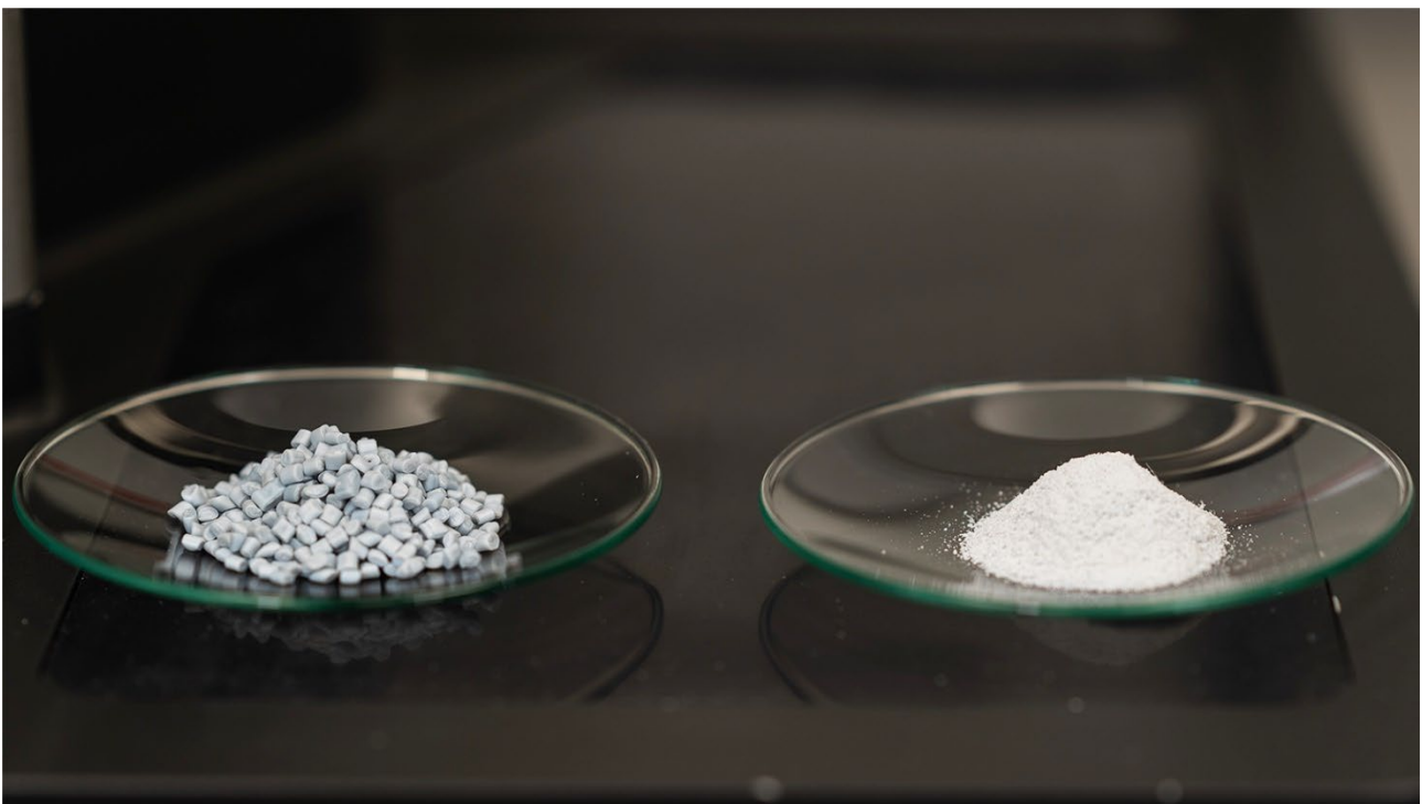
Fig. 1: Plastic sample before and after grinding with the variable speed rotor mill PULVERISETTE 14 premium line
