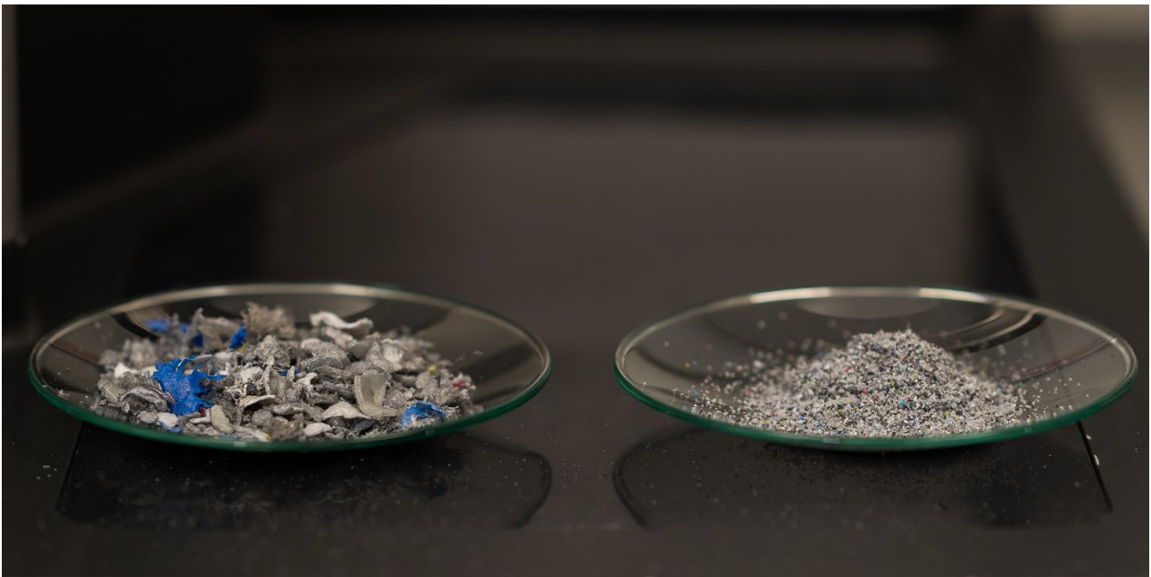
Fig. 2: Plastic waste before and after grinding
