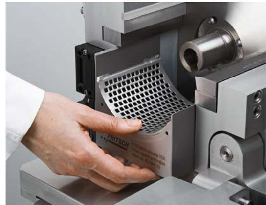
ill.1: Opened grinding chamber FRITSCH Cutting Mill
