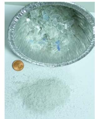
This determination is a wide spread method in the field of chemical polymers. The measured value depends on the particle size. The colour is determined via the white level measuring. But the measured data is greatly dependent on the reflected light and therewith also on the particle size. Therefore prior to the determination of the melt-flow-index and before the measurement of the white level, the samples always must be prepared in a reproducible manner.
