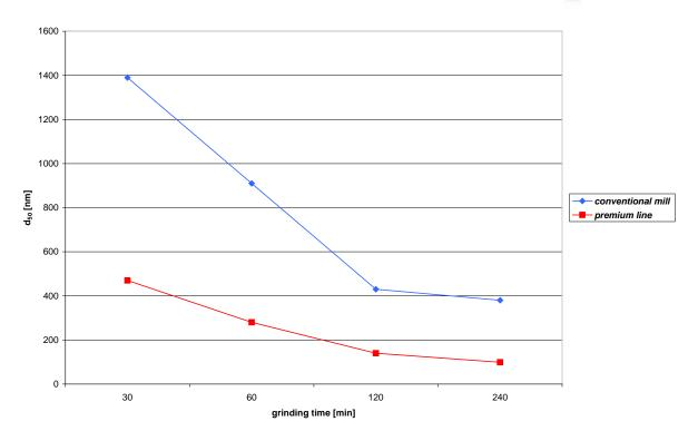
Fig. 1 Comparison of the new premium line with a conventional planetary mill
