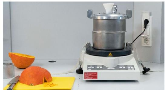
Fig. 1: Pre-cut pumpkin & PULVERISETTE 0 with cryo-box
