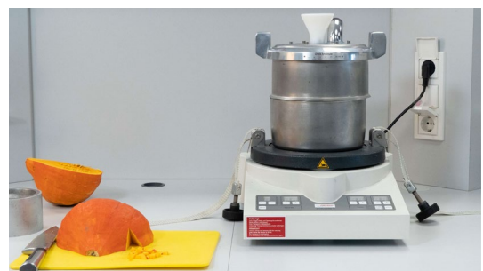
Fig. 1: Pre-cut pumpkin & PULVERISETTE 0 with cryo-box
