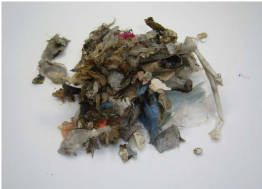
Fig. 4: Secondary fuel prior to comminution
