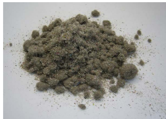
Fig. 5: after comminution – 0.5 mm sieve
