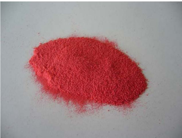
Analytical fineness after milling with PULVERISETTE 14 ,
