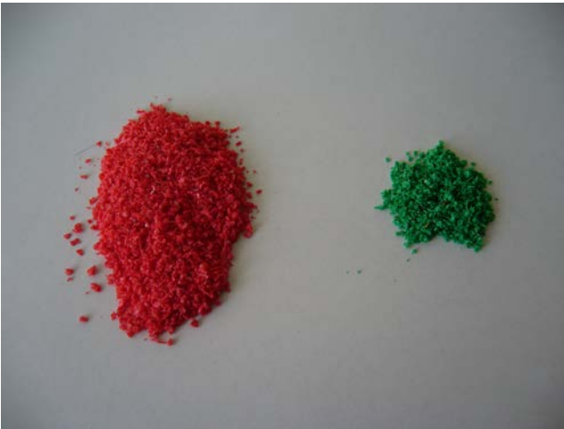
Pre-grinding with PULVERISETTE 19, 2 mm sieve,
