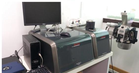
Fig. 3: Particle Sizing ANALYSETTE 22 and a Cross Beater Mill PULVERISETTE 16
