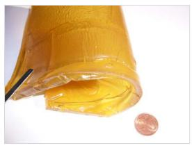
Fig. 1: Rubber slabs prior to comminution
