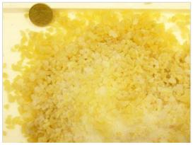
Fig. 2: Rubber processed with dry ice: This processing prevents the granulate from sticking together and it therefore remains free-flowing or pourable.
