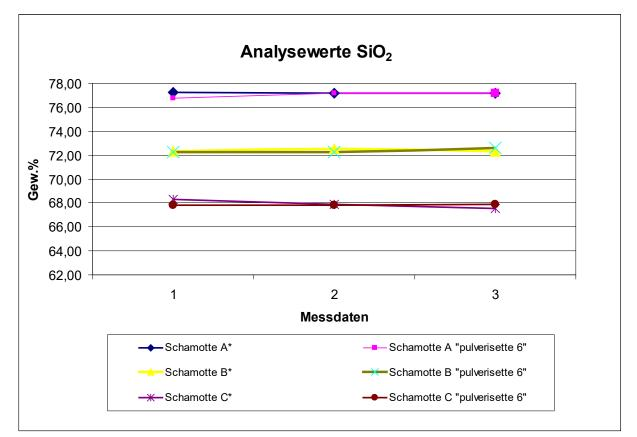
Illustration A: Comparison of the **weight** % of SiO2 of various fireclays from past preparation methods (firing clays A\*-C\*) prepared with the FRITSCH Planetary Mono Mill PULVERISETTE 6 classic line.
