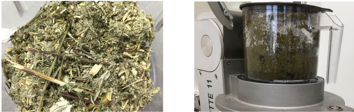
Fig. 3: Dry as well as fresh materials can be comminuted in the Knife Mill PULVERISETTE 11
